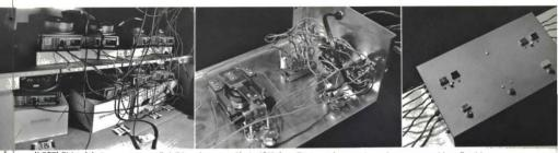
LEFT) Eight of the ten remote-controlled slide projectors used in the 1968 show. The taped-down numbers refer to screen positions. For this temporary set-up, projector boxes were used as stands. (CENTER) Part of the slide control-box interior. Sequencing relay is on the left. The two relays on the right could change slides in up to five projectors. (RIGHT) Theremove-control box ran two banks of slide projectors. Colored lights indicated switch positione in the dark.
